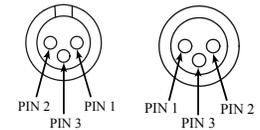
**Power Control and Trigger Connectors**
